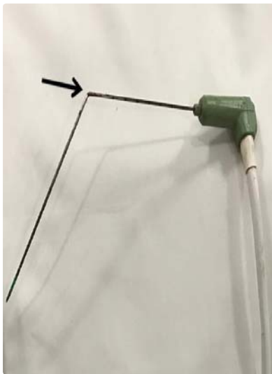
Figure 5A: Partially-fractured probe (arrow).
