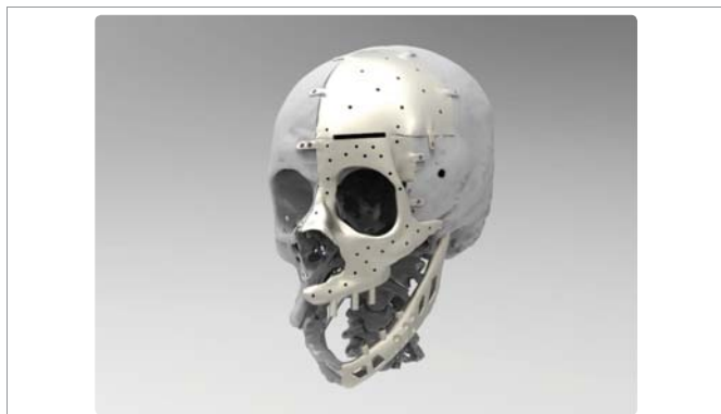
Figure 1D: Computer Assisted Design (CAD) of the facial implant.
