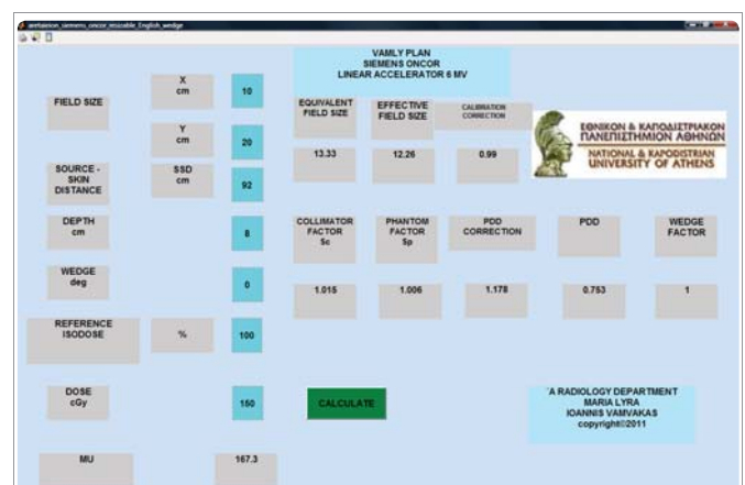
Figure 1: The VAMLY plan graphical user interphase. At this example user inputted for field size (10 cm x 20 cm), SSD (92cm), depth (8 cm), wedge filter (0 for open field), reference isodose (100%) and dose (150 cGy). Then user pressed the green "CALCULATE" button and the MU's were displayed (167.3). Also all the required parameters for the specific calculation were displayed (Sc, Sp, PDD, wedge factor and correction factors for calibration and SSD)
