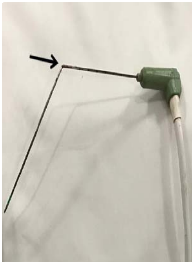
Figure 5A: Partially-fractured probe (arrow).
