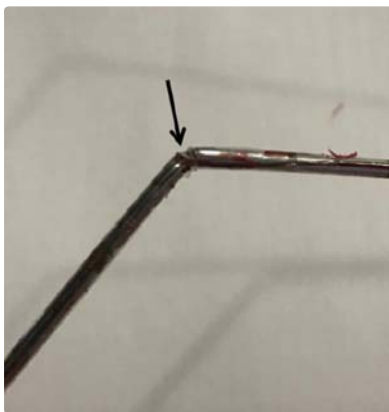
Figure 5B: Close-up of the fractured portion of the probe (arrow).
